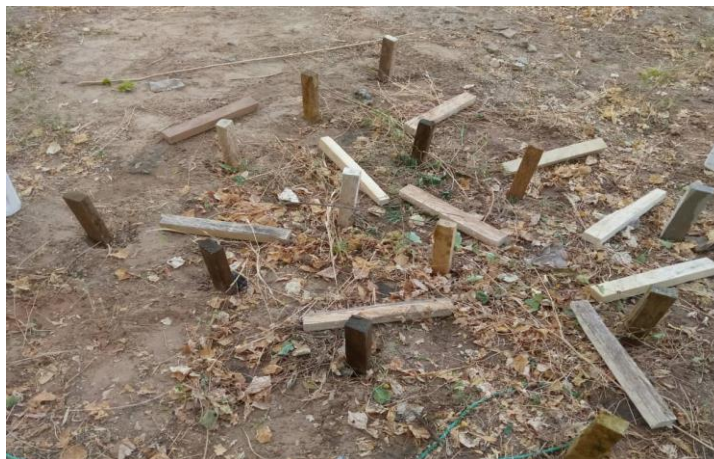
Photo 1: Graveyard experiment on Obeche and Oro timbers
