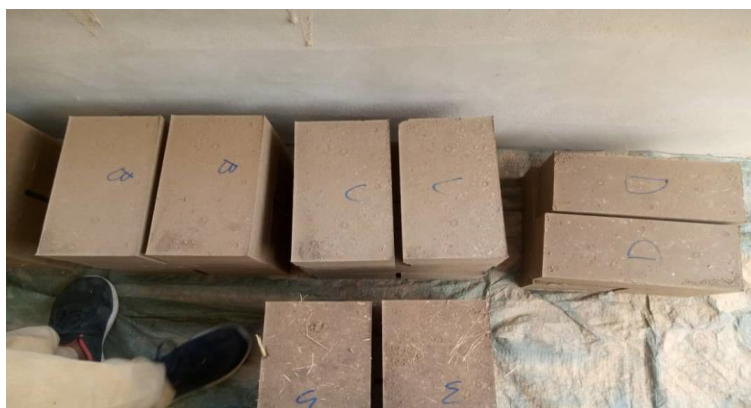
Photo 2: Compressed stabilized mud brick samples
